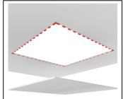
Be aware of any obstructions or trusses where you want to located LED panel. Mark & cut plaster using template provided using a plaster knife
